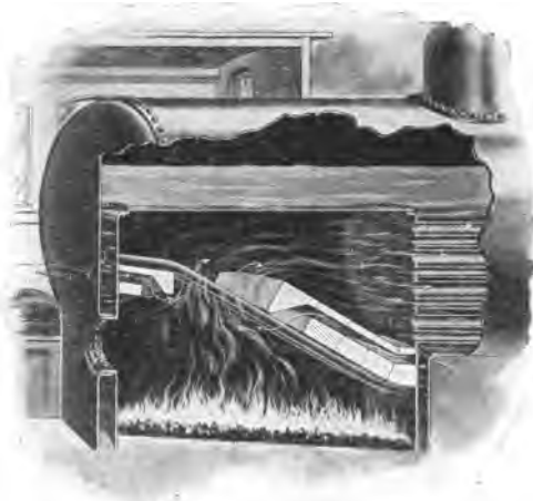
Fig. 15. Wade-Nicholson Hollow Arch Installed in Locomotive Boiler. The Water-Tube Supports Here Shown are Sometimes Omitted.
